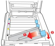
**13.** Pressing gently down on the cartridge to ensure that it is firmly seated, push the colored lever (1) towards the rear of the MFP. This will lock the cartridge into place and release toner into the image drum unit.
